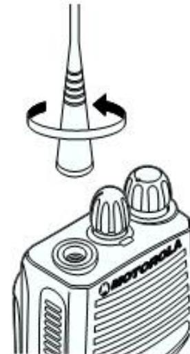
Turn the antenna counter-clockwise to remove it.
