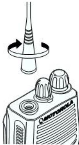
Turn the antenna clockwise to attach it.
